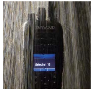
Heavy Rain Test
